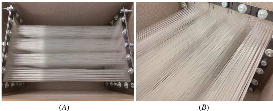
FIG. 1 The views of completed formwork. (A) Top view of the completed formwork. (B) The view of the metal frame with fibers.
