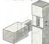
INTERLOCKING MORTISE & TENON JOINT WITH CAR TENON
