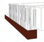
Vertical Orientation Screens for Microclimate Regulation At the end of the building, orientation screens for the southern side, combined with vertical fins, are installed to optimize the building's microclimate. They contribute to reducing a cooler and more comfortable microclimate in the surrounding outdoor space.
