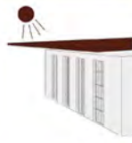
Shading Meets Overhangs The roof overhangs, made of recycled metal, are dimensioned to block direct summer rays, preventing overheating of interior spaces and reducing the need for artificial cooling.
