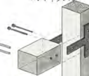
SQUARE CUTS WITH STEEL PLATES * THROUGH BOLTS
