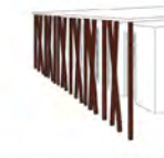
Solar Screens with Bars For the south-facing façades, used in some cases also on the north, the overhangs integrate sun-shading ribs that filter light and create dynamic shadow patterns. These elements respond to the quality of natural lighting while limiting heat buildup during the hottest hours.
